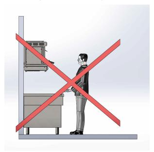
The Beef-Star has an air cooling system. Under no circumstances may the openings for supply air (in the floor) and exhaust air (side in the lid) be covered or delivered.
