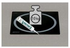
Fill the side joints between ceramic glass and work surface with sufficient pactan. Easily run over material.
