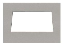
Making the cut-out in the work surface according to Built-in drawing. **Glass dimension + all-sided 3mm joint**
